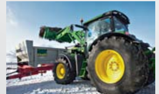
The H310 is a more compact loader, ideal for front loader applications in small places. The lift capacity of the H310 is up to 1.85 t and 3.8 m height.*
