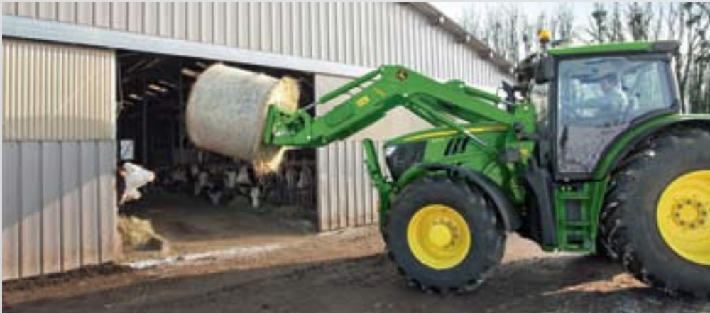
The H340 and H360 are the right choice if you spend a lot of time during the year loading. The lift capacity of the H360 is up to 2.0 t and 4.4 m height.*
