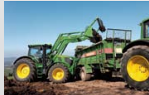
The H380 is designed for years of heavy duty work with a lift capacity of up to 2.15 t and 4.5 m height.*
