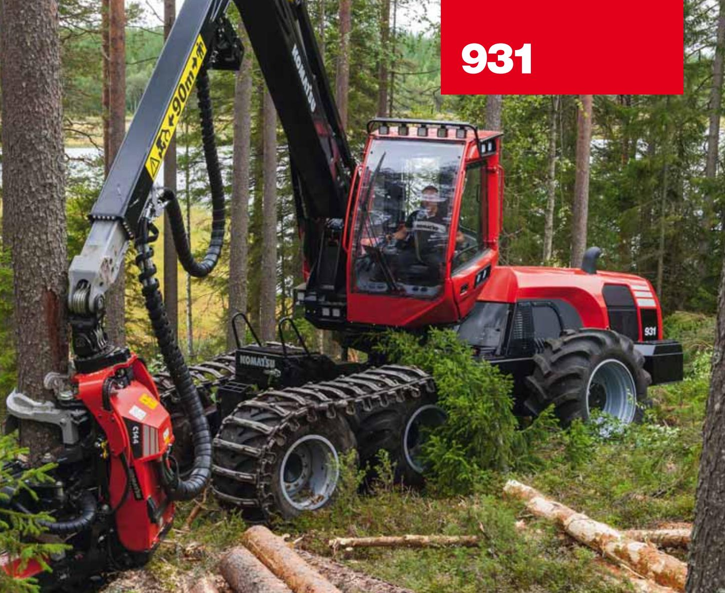
the lifting power you need. What's more, the smart pressure and flow optimisation means that you can do several things at once, such as slew and feed, with full hydraulic power and maintain a considerably higher work rate. To this we can a full 360 degrees of cab rotation that enables you to process more from the same spot, which optimises forwarding.
