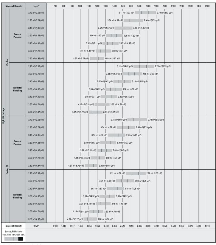
**Note:** All buckets are showing Bolt-On Edges. Material Handling buckets are flat floor buckets.
