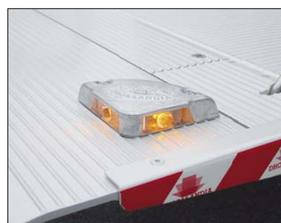
S090 Platform lights mounted onto the platform
