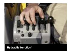
The hydraulic system in the L50E is prepared for installation of a third hydraulic function. The separate third hydraulic function, with its control lever and additional lines, can easily be installed to further increase the machine's flexibility.
