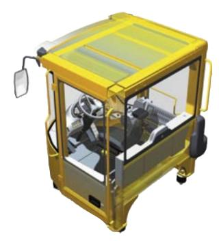
the operator can operate steering, forward, reverse and kick-down with controls on the left armrest. At any time, the operator can switch between steering with the steering wheel and CDC, which helps to minimize tiring and repetitive movements. This gives the operator the possibility to vary operating modes, thus combatting fatigue and static muscle strain.
