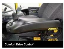
Significant reduction of repetitive and tiring steering wheel movements with CDC. Comfortable operation of steering and shifting with user-friendly controls in the left armrest.
