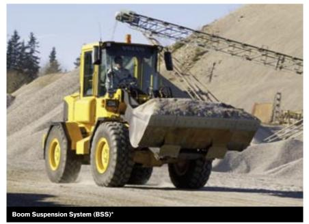
Gas/oil accumulators connected to the lift cylinders effectively reduce vibrations that often occur when running over rough ground. Boom Suspension System gives faster cycle times, less material spill and improved operator comfort.
