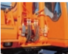
Boom and arm hose rupture protection valve
