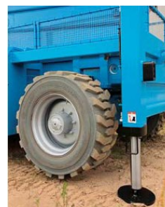
Automatic self-levelling outrigger system and oscillating axle
