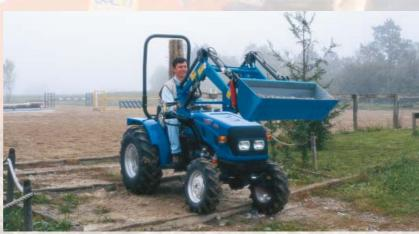
litres. The lifting capacity at the link arm ends is 700 kg. There is also the optional electronic lift with position, draft, intermix and maximum lift height control.
