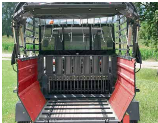
Smooth sides, powerful chain-and-slat conveyor – the smaller Vicon models are true load masters, too.
