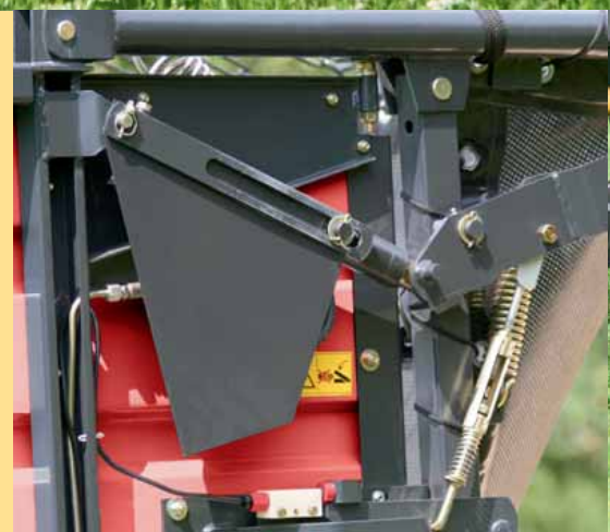
The tailboard features standard hydraulic operation.
