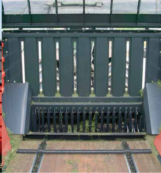
Smooth interior sides guarantee positive crop feed to the rear.
