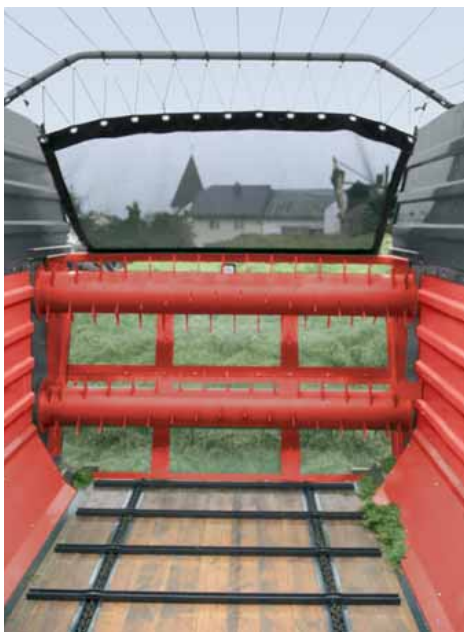
Two discharge rollers unload the crop to an even mat.
