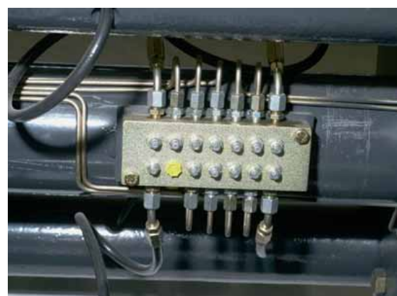
Service made easy – all grease points are grouped in a bank.
