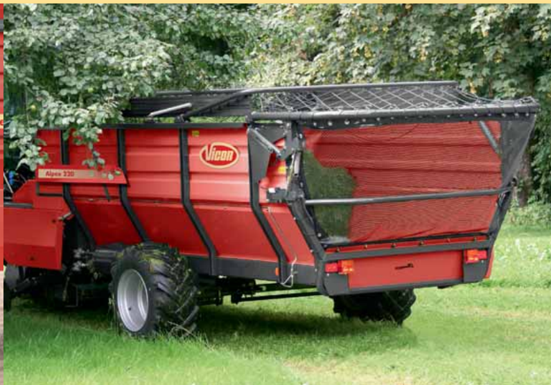
Hydraulic hay extensions for all Alpex 220-Feedex 360T models. Convenient adaptation of load height from tractor cab.
