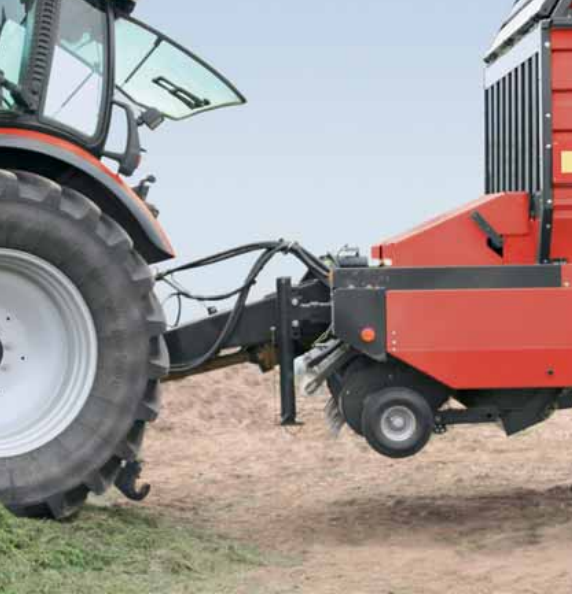
The hydraulic artic drawbar provides a 600mm ground clearance for ultimate stability on the clamp.
