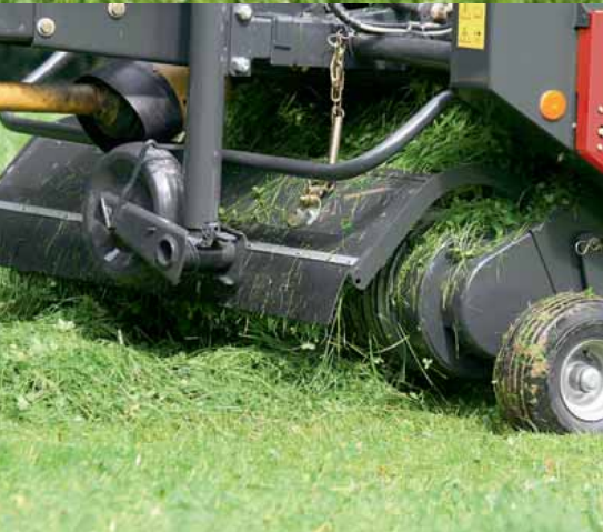
The standard baffle plate ensures a uniform crop flow into the machine.
