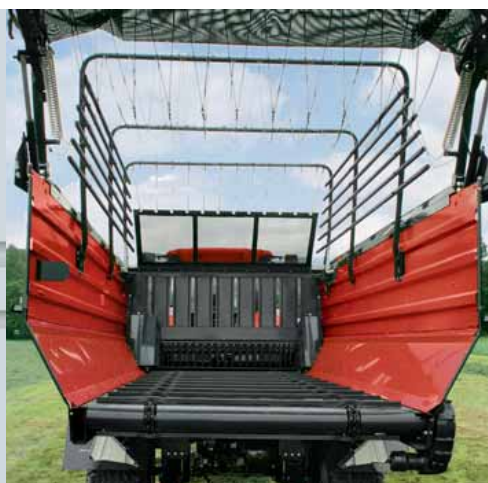
Smooth interior walls and foldable hay extensions.
