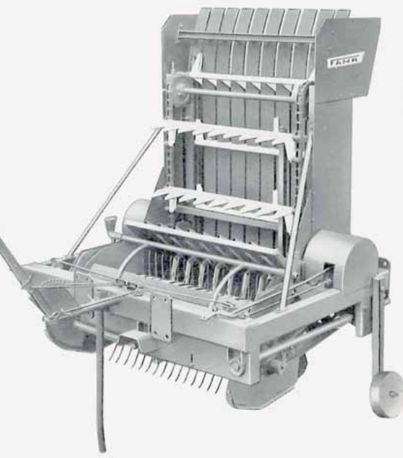
The feeder unit on the first forage wagon. This design cut harvest time to a tenth of the time previously required.
