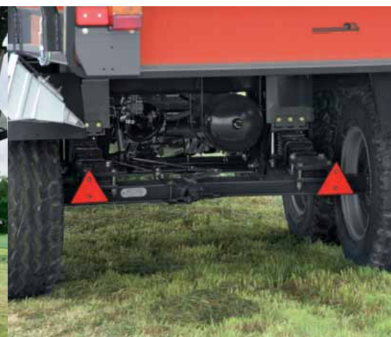
The stable and spring-loaded tandem axle provides high driver comfort (Feedex 360 T).
