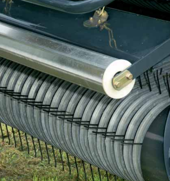
The roller crop guard is standard specification on all models from Feedex 300.
