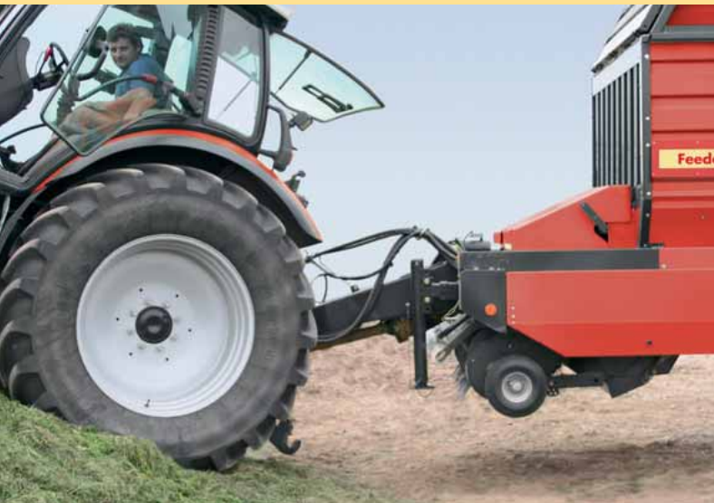
Hydraulic artic drawbar is available for all Alpex 220-Feedex 360 models. High ground clearance of up to 600mm provides for stability on ramps and clamps.
