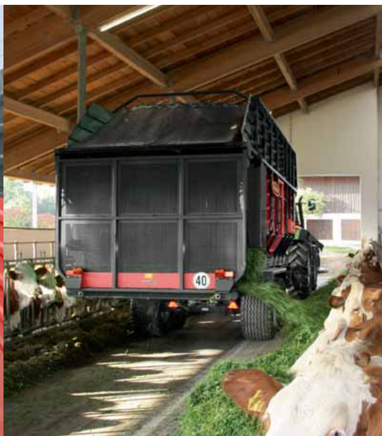
The bi-directional cross conveyor allows for right and left hand discharge, saving time and money when daily rations include fresh-cut forage.
