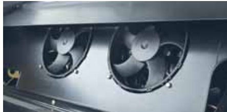
Clean knotters add to exceptional knotter performance. Knotter fans are standard, and the new round knotter compartment shielding further increases air flow for improved fan efficiency.
