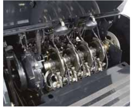
New curved knotter shielding offers great access to knotters and knotter fans for easy twine threading and maintenance jobs.
