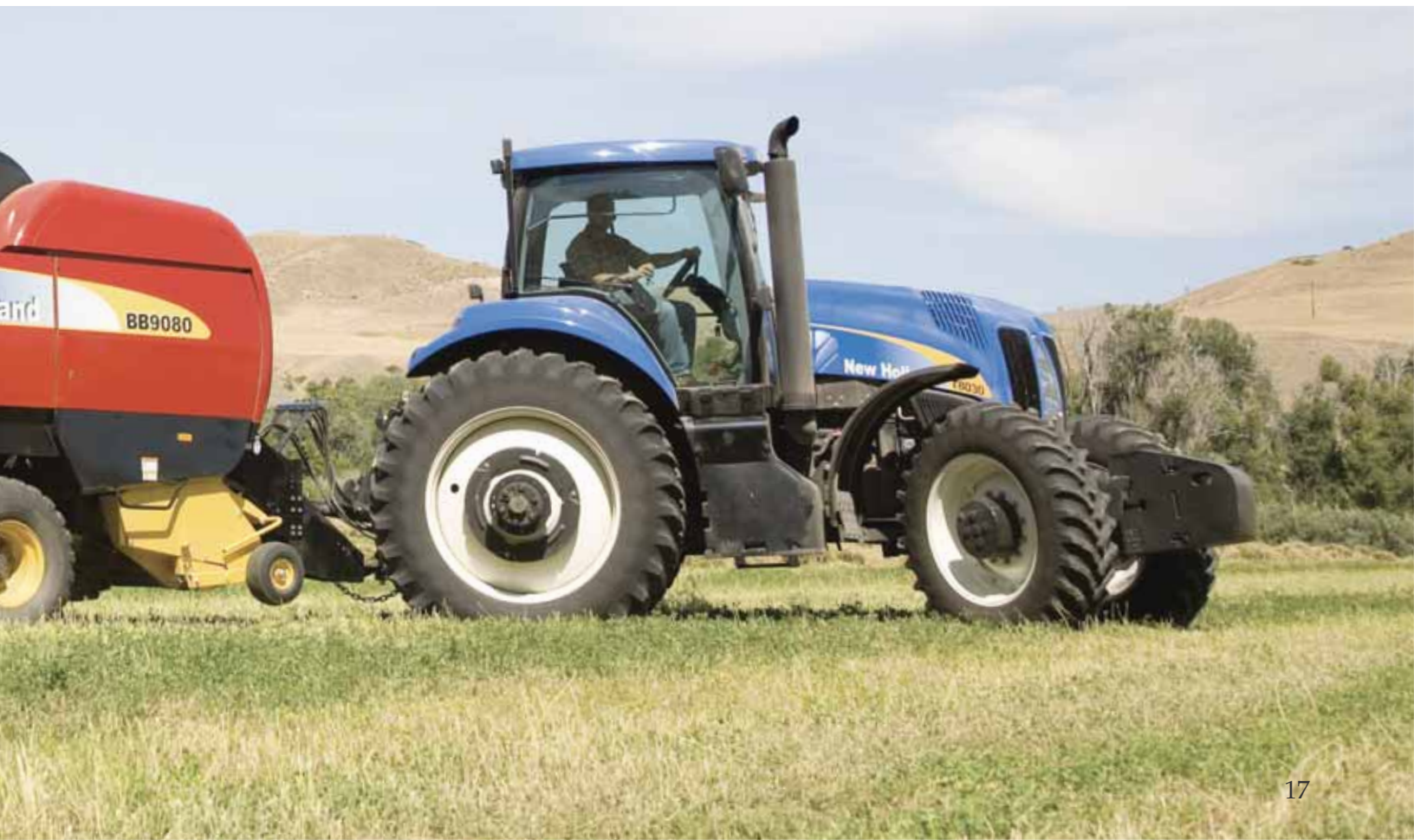
The tandem axle helps smooth the ride over rough terrain or for higher-speed road travel.
