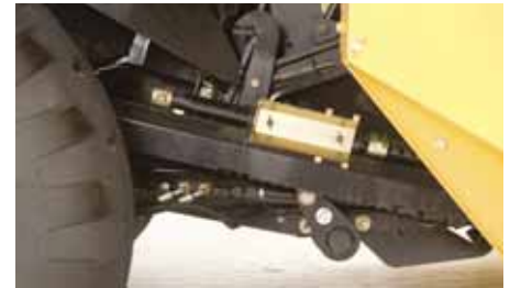
An adjustable flotation spring allows for easy, tool-free adjustment of the SuperSweep™ pickup flotation range for smooth field performance.
