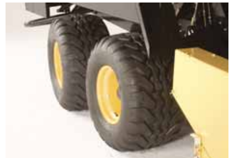
The tandem axle helps smooth the ride over rough terrain or for higher-speed road travel.
