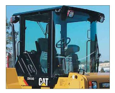
**Seat.** The comfortable and durable seat has adjustable fore/aft position, suspension stiffness and flip-up arm rests with a 76 mm wide retractable seat belt.
