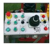
The control panel of the basket provides improved clarity oas far as lift movements are concerned. The compact panel also includes a 230 V standard outlet.
