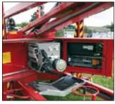
The electric and hydraulic cabinets of the lift are easily accessed. This feature provices user-friendly access for adjustment and repair work.
