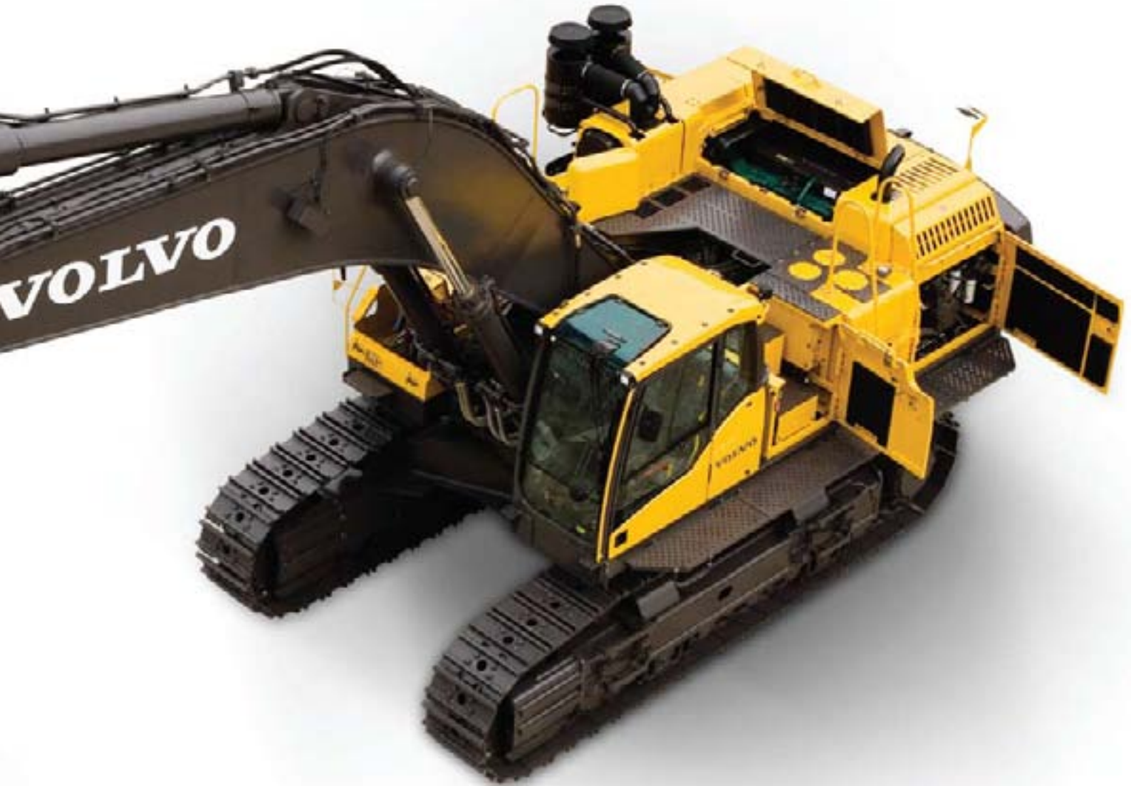
• Simplified, centralized lubrication points.
