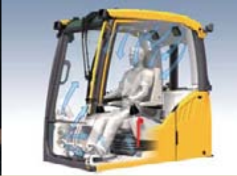
• Industry's highest heating/cooling capacity with 14 vents.
