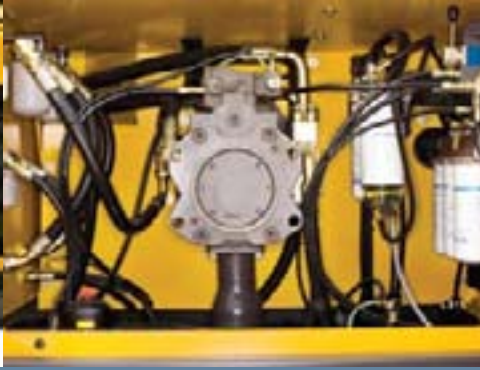
• Easy access to hydraulic pumps and filters.
