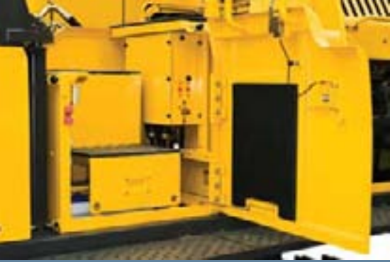
• Simplified, centralized lubrication points.
