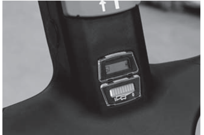
Clear display of battery condition and operating hours
