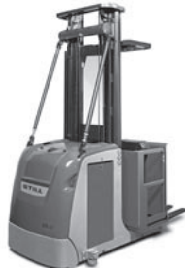
EK-X telescopic lift mast height 2,400/2,900 mm
