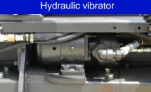
The compaction system is hydraulic vibrator. It is possible to change compacting intensity according to a kind of material.
