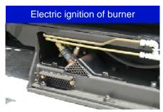
For easy handling the screed is equipped with an electric ignition of the gas burners.
