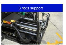
High strength 3 rods support controls shakiness of the screeds.
