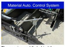
The sensing paddle behind the tractor in respective right and left sides automatically control the conveying volume of Asphalt mix gearing to the bar feeder and spreading augers
