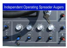
Independent spreading is available during automatic material spreading mode. Speed for the bar feeder and spreading augers are proportionally solenoid controlled so that it is able to set the best feeding volume and material lateral distributions easily and an independent left and right operation as well as to select forward and reverse auger revolutions.
