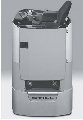
Narrow chassis contour for high manoeuverability in confined spaces
