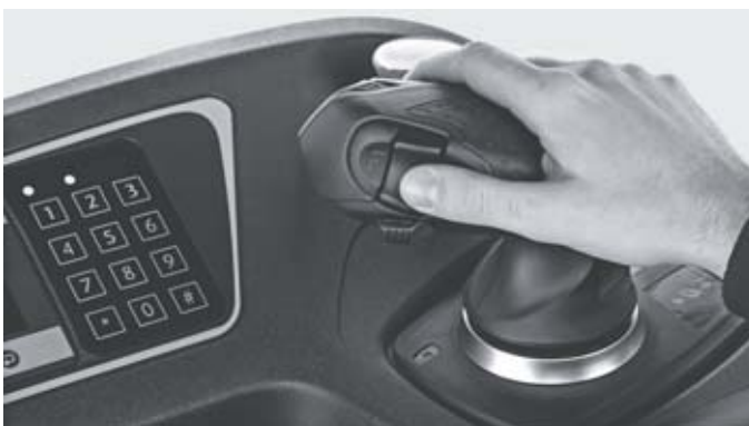
Optional Joystick 4Plus for lift, lowering and transmission control without having to change hands
