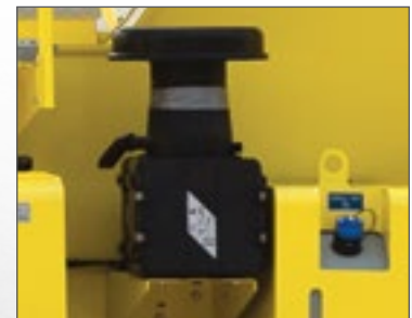
Tier 4 Final integrated pre-cleaner and air filter
