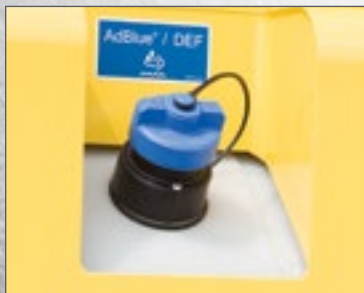
Diesel Exhaust Fluid (DEF) tank
