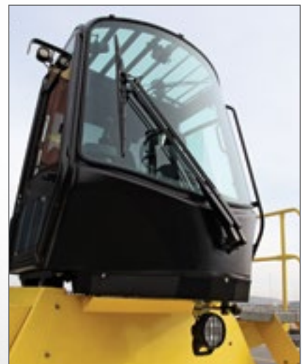
Cab offers large windows fitted with tempered safety glass, with excellent all-around visibility.
