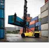
Nine models available, four single container handlers up to 8 high and five double container handlers up to 9 high. The Hyster on-demand load sensing system lowers fuel consumption and extends component life.
