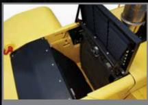
Hinged cover enables easy serviceability access to radiator cooler
