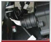
Standard profile Deutsch pin connectors, IP64 compliant
