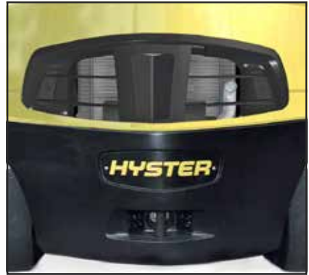
Counterweight venting improves airflow
