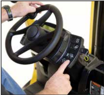
Infinitely adjustable steer column
