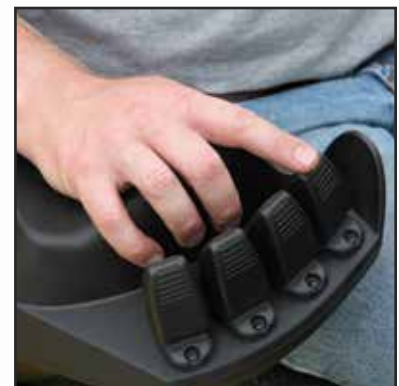
TouchPoint mini-lever electro-hydraulic controls
