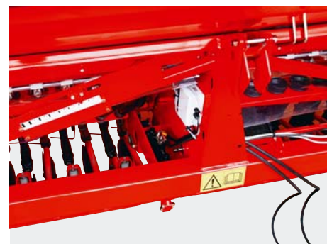
Lower stop positioned for seed depth of 8 cm and 1 cm respectively.
