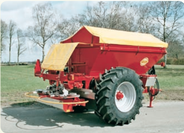
K45 with 16.9 x 30 tyres, 12-36 m fertilizer equipment, hopper extension, cover over spreader system and hydraulically-controlled dosing.
