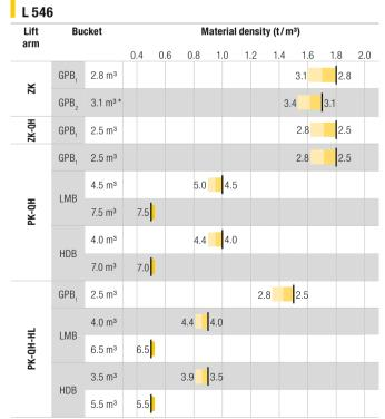
$<sup>^{\</sup>star}$  Toothed buckets, hydraulic quick hitch and additional hydraulic circuits are not approved for rehandling application.
