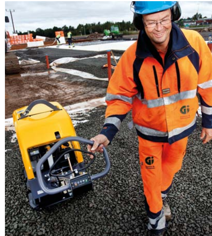
The single hydraulic control valve makes changing direction fast and easy.
