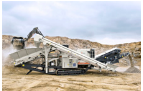
The Lokotrack® LT200HPS™ cone plant can be equipped with either one or two-deck detachable screens.
