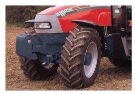
The specially sculptured front axle carrier allows the MC Power6 to perform one of the tightest turning circles in the industry.
