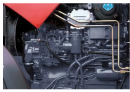
The engine service intervals are 500 hours resulting in lower operating costs. A rear hinged tilting bonnet allows complete engine component access with a handy side opening panel for quick, effective air filter servicing.
