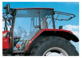
The low profile cab option is ideal when operating around low roof buildings. This option provides all the deluxe comforts of the high roof version and is available with air conditioning. A roof window provides exceptional visibility particularly during front loader operations.
