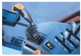
The MC Power6 comes with the well proven 4-speed Powershift and smooth directional change of the Power shuttle. The optional Autospeed transmission further improves operator efficiency by allowing the driver to shift through the Powershift speeds and ranges at the touch of a button.
