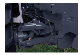
With rigid or optional Independent Front Suspension, both having the choice of internal wet disc brakes, maximum productivity and comfort are achieved.
