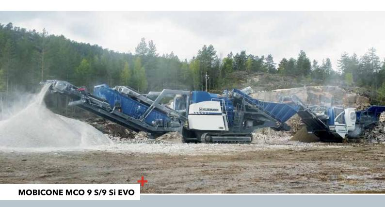
The MCO 9 S EVO has a more powerful hydraulic drive than the MCO 9 EVO and a larger running gear and chassis. As an option, it can also be equipped with a secondary screening unit (single-deck vibrating screen) with return conveyor. This permits an endless material loop, thus guaranteeing a qualified final grain size. The oversize grain can be discharged optionally at the side via the return conveyor that can be swivelled out up to 100°.
