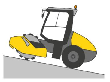
Master up to a 60% gradient thanks to the wheel motors.
