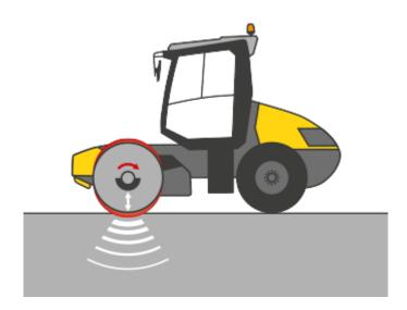
Compaction through vibration Vibration for high compaction depth. **RC50** and **RC50p**
