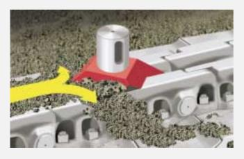
The patented track cleaning and guide system is an effective safeguard against dirt. While the unit is travelling, the tracks are automatically cleaned. The wedge shape of the cleaning shoe dislodges the dirt sideways out of the tracks, preventing build-up at the idlers and sprockets. Track wear is significantly reduced, the track tensioning system has less work to do and the tracks are prevented from slipping off.
