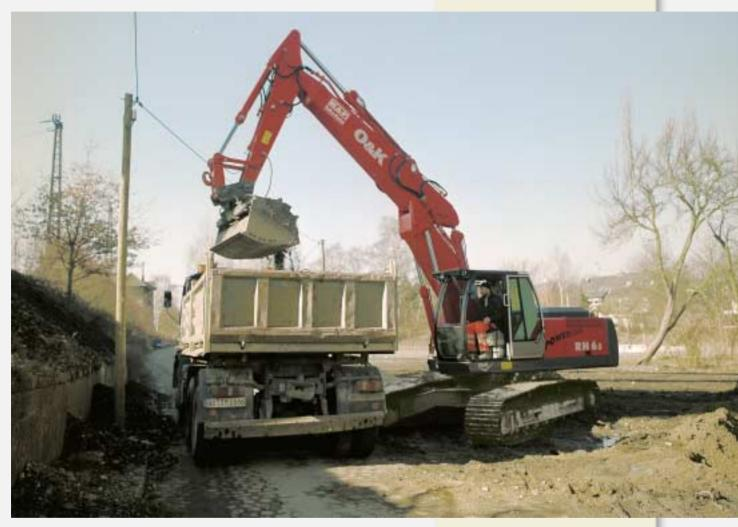
Service weight 20.6 – 23.1 t Engine output 113 kW Trenching buckets up to 1.45 m³ (SAE)
