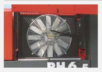
The cooling system on O&K crawler excavators has been completely reengineered. Cool air is taken in behind the control valves for significantly less dust contamination, compared with outside air intake. In order to cool the engine, the intake air is routed through the engine compartment for additionally reduced ambient temperatures. An external combined radiator ensures heat exchange. The air is exited upward.
