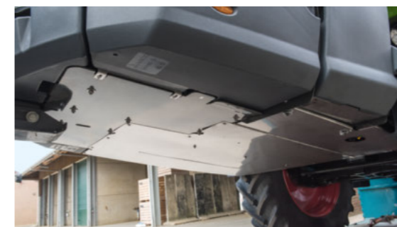
The high ground clearance of up to 85 cm, and the smooth undercarriage with no sharp edges guarantee minimal damage to plants.
