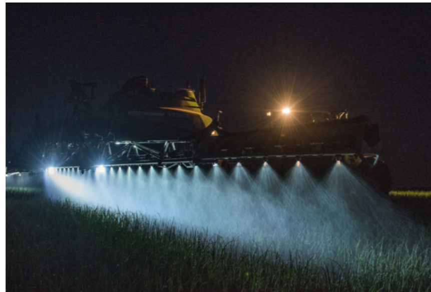
■ LED headlights for an optimal view of the nozzle fans. 2 or 4 blue LED main lights are also available as an option. Headlights are fitted in front of the nozzle to protect against deposits.
