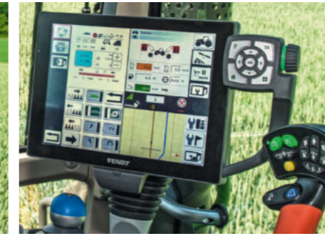
The Fendt Varioterminal gives you a perfect overview of your Rogator 300 with all relevant machine functions, SectionControl including coverage map, as well as other configurable functions.
