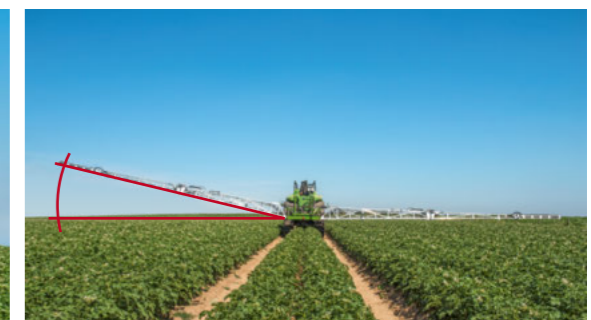
The ground contour or crop can be used as a reference for height control to precisely adjust the boom to suit your crop. Hybrid control is also possible.
