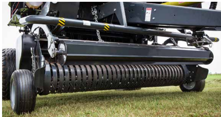
Large diameter roller crop press facilitates crop flow at high intake speeds.
