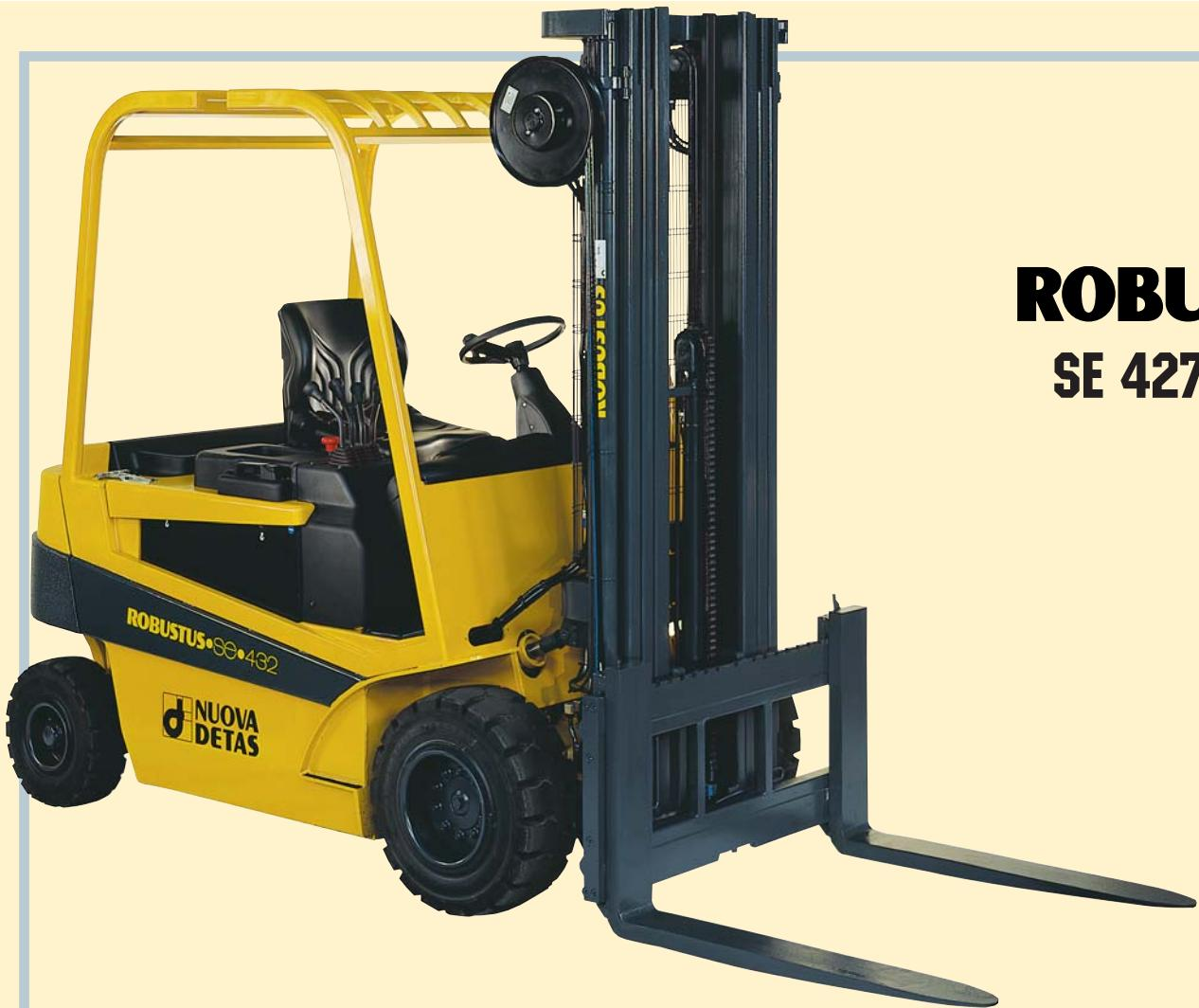
The **SE 427-432 AC** series trucks are of an extremely new and innovative line, differing from conventional models. The compact form, excellent load distribution and low centre of gravity guarantee exceptional over capacities under any operational condition.
