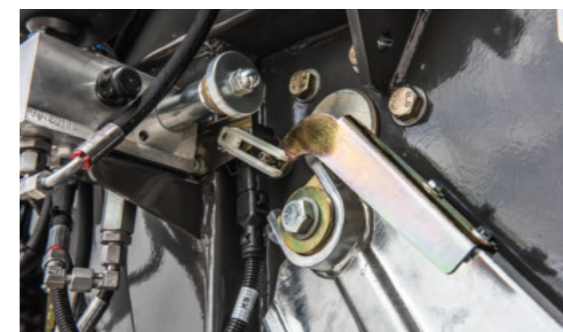
The drawbar position control ensures that the set opening angle of the pick-up is automatically sustained and controlled. This guarantees an even and constant crop flow without constriction, and clean raking even in hilly terrain.
