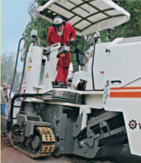
The rear right-hand suspension unit is normally swivelled outwards.
