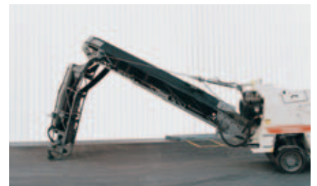
It can also be folded up just as easily to reduce the overall machine length.
