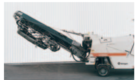
Shorter trailers can be used to transport the machine when the belt is folded up.
