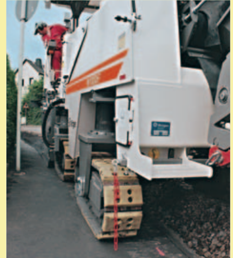
So the machine can mill round obstacles without interference.
