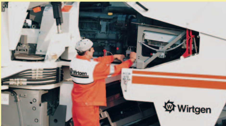
The engine hood opens wide to permit easy access to the engine and to the handful of maintenance and inspection points.
