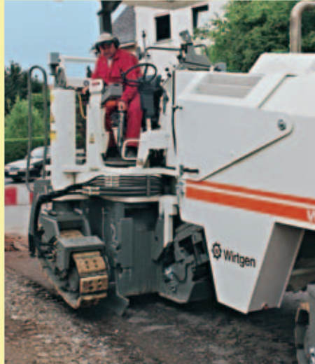
If space is limited, this unit can be hydraulically swivelled in front of the milling drum.
