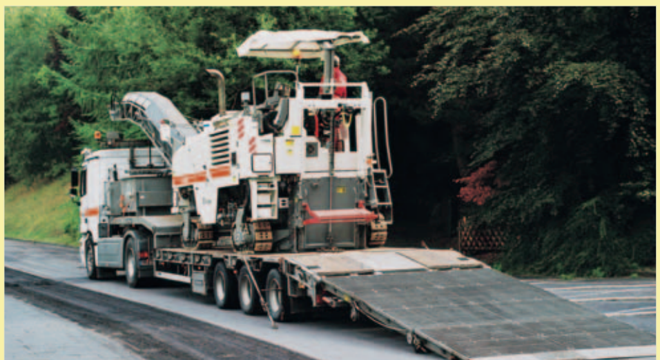
Quickly and safely: the canopy roof is lowered hydraulically and the machine is securely lashed after being loaded onto a low-bed trailer to be transported to the next site.
